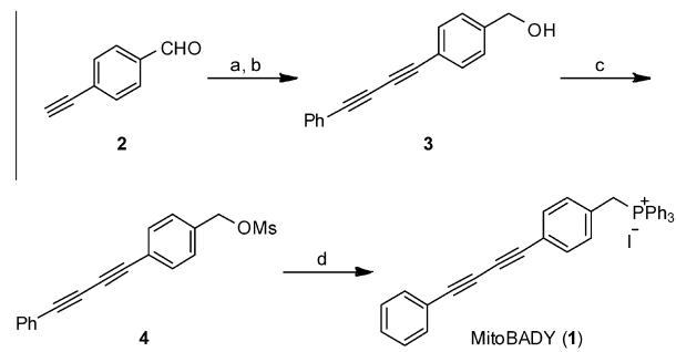
**Scheme 1.** Synthesis of MitoBADY. Reagents and conditions: (a) Ethynylbenzene, CuI, NiCl<sub>2</sub>·6H<sub>2</sub>O, tetramethylethylenediamine, air, THF; (b) LiAlH<sub>4</sub>, THF, 0 °C, 52% for 2 steps; (c) MsCl, Et<sub>3</sub>N, CH<sub>2</sub>Cl<sub>2</sub>, 76%; (d) PPh<sub>3</sub>, NaI, MeCN, 75 °C, 95%.
