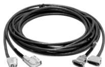
**Camera Power & Signal: 2-D OMA V 1MHz/5 MHz systems only.** This cable assembly (6050-0313) consists of two cables that interconnect the Camera Power and Camera Signal connectors on the back of the ST-133 with the mating connectors on the back of the detector. The Camera Power cable has DB-15 Male connectors with locking screws at both ends. The Camera Signal cable has DB-40 Male connectors with slide-latch locking mechanisms at both ends.
