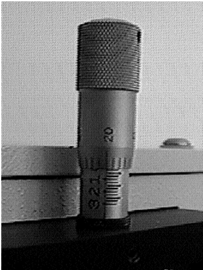
Slit Width Setting: 200 Micrometers (0.200mm)
